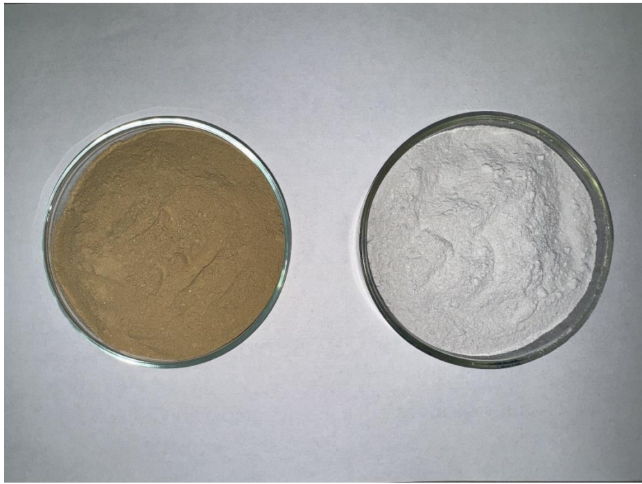
Figure 2 - Obtained purified white carbon black (technology of obtaining rare and rare-earth metals and white carbon black from the weathering crust ores of the Kundybay deposit)
